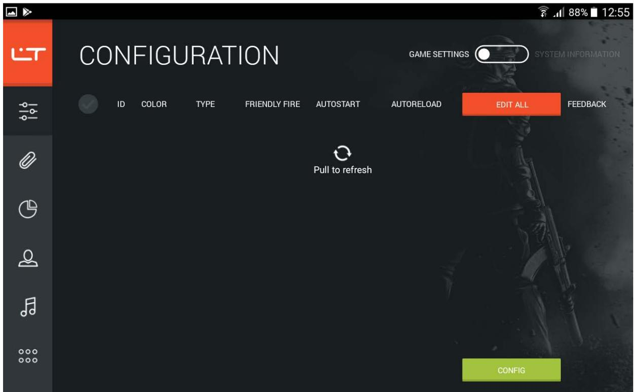
Connect playsets by launching them in configuration mode. In the application drag the update icon down. Equipment search will be performed and after some time a list of connected devices will be formed.
